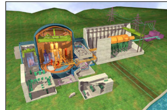
AREVA US EPR (1600 MWe)
